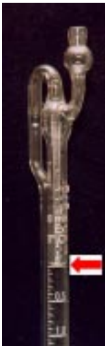
Step 14: ...till the level of sodium thiosulphate is at zero
