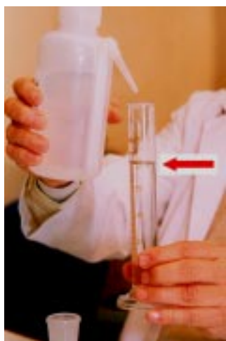
Step 3: Carefully measure 50 ml of double distilled water with a measuring cylinder
