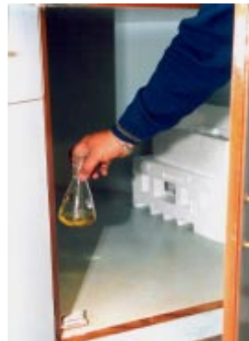
Step 15: After 10 minutes, take the flask out of the dark...
