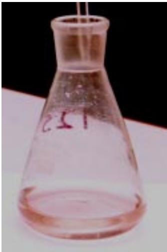
Step 19: Continue titration till the solution colour starts fading...
