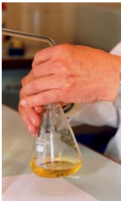
Step 16: Titrate the solution in the flask with the sodium thiosulphate
