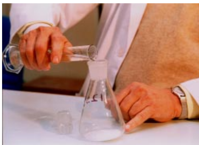
Step 4: Pour the 50 ml of double distilled water into the conical flask
