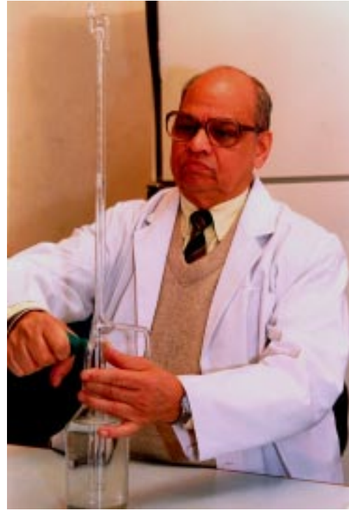
Step 13: ...fill the burette tube with 0.005N sodium thiosulphate, with a pumping action...
