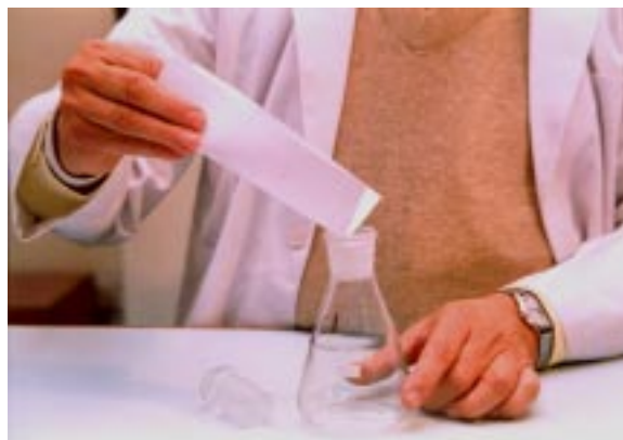
Step 2: Carefully pour the 10 grams of salt into a 250 ml conical flask, which has a stopper
